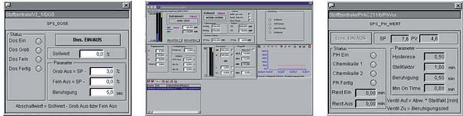
The faceplates for motors, controls and analog value displays contain all plant-relevant data. For example, test-point-relevant alarms and analog value diagrams are displayed. Alarm limits can be adjusted for selective plant supervision. The shutdown of valves and motors is indicated in plain text along with the current status.
