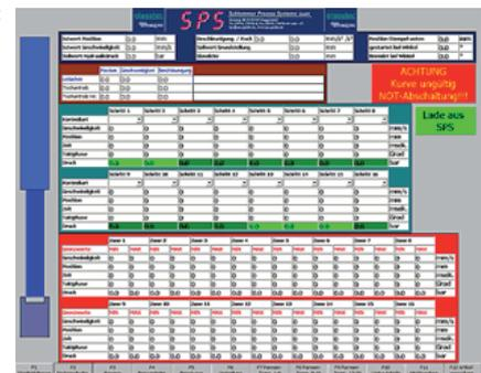
The recipe management is included in the pictures "production setup" and "article management" of the visualization. Every adjustment of a produced article can be saved on hard disc or on a server. If such an article should be produced again, the adjustments must only be loaded again from the recipe file. All parameter, which the customer needs, can be saved. It doesn't matter if the data are general information or cams with thresholds.
